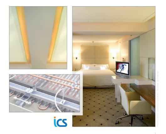
The climaBOARD® Segel is a seamless plasterboard system. The cooling sail hangs beneath the actual ceiling and can be placed in specific points. Cooling load removal takes place by means of approximately 40% radiation and 60% convection. The surface can be finished according to your individual requirements and tastes and is suitable for both Q2 and Q3 surface qualities.
