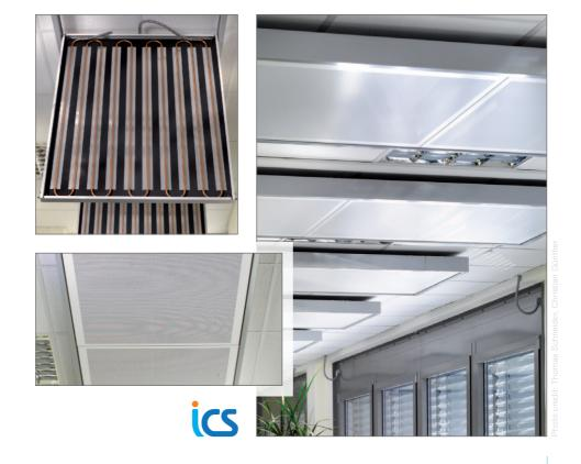
The climaTILE® Segel is an acoustic cooling ceiling of metal cassettes which removes sensitive heat loads. The cooling sail hangs beneath the actual ceiling and can be placed in specific points. Cooling load removal takes place by means of approximately 40% radiation and 60% convection. The surface of this ceiling is available with either a smooth or perforated finish, depending on your requirements.
